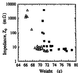
Fig. 3. Relationship between impedance  $Z_0$  and weight for used cells: (■) manufacturer A, and (△) manufacturer B.
