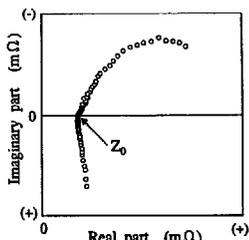
Fig. 4. Typical Cole-Cole plot for a Ni/Cd cell.
