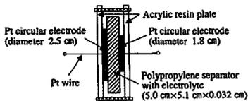
Fig. 1. Experimental setup for measuring the impedance of a separator.
