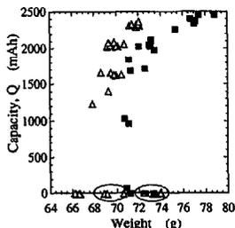
Fig. 2. Relationship between cell capacity and weight for used cells: (■) manufacturer A, and (△) manufacturer B.
