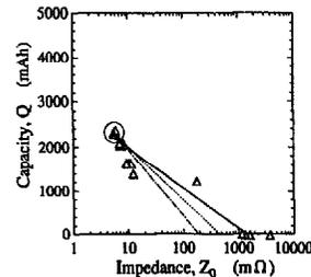
Fig. 12. Relationship obtained from used-cell data and relationships obtained from model-cell data: (—) from used-cell data of manufacturer B; ( $\cdots$ ) from model-cell data of manufacturer A: C and D size (overlapped); (---) from model-cell data of manufacturer B: D size.
