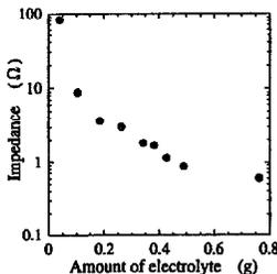
Fig. 13. Dependence of separator impedance at 1 kHz on amount of electrolyte.
