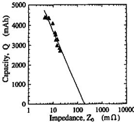
Fig. 9. Relationship between cell capacity and  $Z_0$  for D-size model cells made by manufacturer B.
