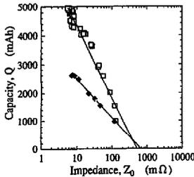
Fig. 8. Relationship between cell capacity and  $Z_0$  for model cells made by manufacturer A: ( $\square$ ) D size, and ( $\blacklozenge$ ) C size.
