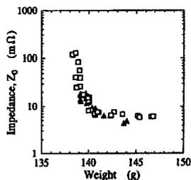
Fig. 7. Relationship between  $Z_0$  and weight for D-size model cells: (□) manufacturer A, and (△) manufacturer B.
