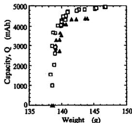
Fig. 6. Relationship between cell capacity and weight for D-size model cells: (□) manufacturer A, and (△) manufacturer B.
