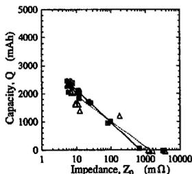
Fig. 5. Relationship between cell capacity and  $Z_0$  for used cells: (■...■) manufacturer A, and (△...△) manufacturer B.
