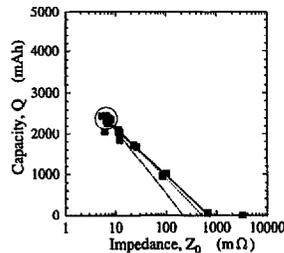
Fig. 11. Relationship obtained from used-cell data and relationships obtained from model-cell data: (—) from used-cell data of manufacturer A; ( $\cdots$ ) from model-cell data of manufacturer A: C and D size (overlapped); (---) from model-cell data of manufacturer B: D size.
