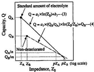
Fig. 10. Derivation of quantitative relationship between  $Z_0$  and capacity: (—) model cells, and (---) used cells.
